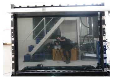
Setting up the camera in preparation for an experiment on the Artificial Volcanic Fissure machine, to study and model how lava erupting out of volcanic fissures is controlled by the shape of the crack it is moving through. At the geology department in the University of Otago
